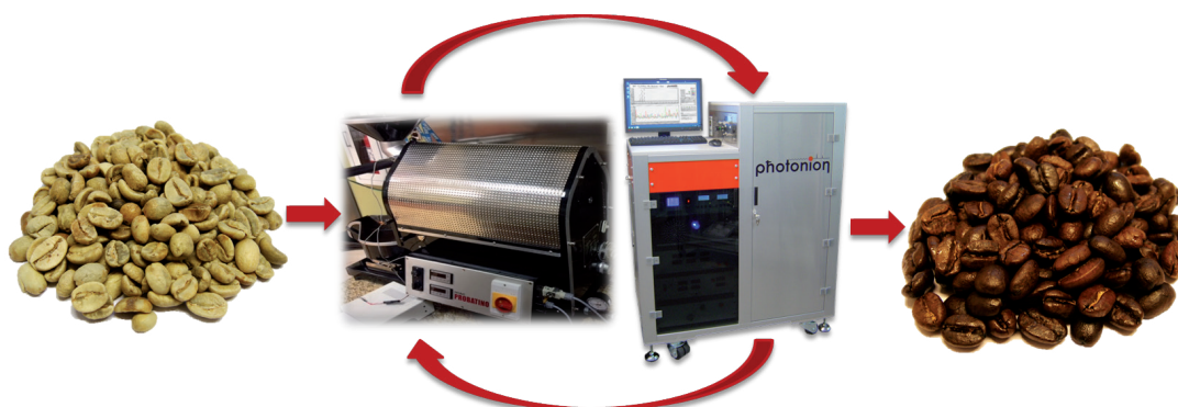
Figure 1: Schematic representation of the project goal as a real-time measurement and control system for coffee roasting.
