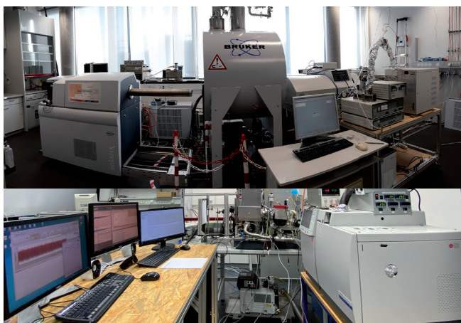
Figure 4: High-resolution MS laboratory in the Research Building LLM of the University of Rostock where the Chair of Analytical Chemistry/JMSC operates an FT-ICR MS System. Top: The 7 T FT-ICR MS exhibits two carts allowing MALDI, ESI, GC-/TA-APCI, APPI, APLI ionization experiments. Bottom: An Orbitrap for photoionization of gases and particles is developed in the framework of the AerORBI EU Project.
