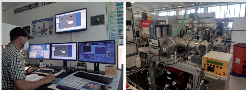
Some impressions of the first measurement campaign performed at the LKV in Rostock. (Left) Central control unit for the experiments on the ship engine. (Right) Instrumentation for online measurements of gaseous and particulate emissions.
