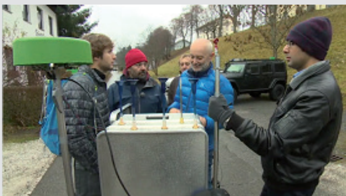
Measuring- and recording device for capturing particle matter of different sizes, particle number concentrations, aerosol particle size distribution, black and brown carbon.
