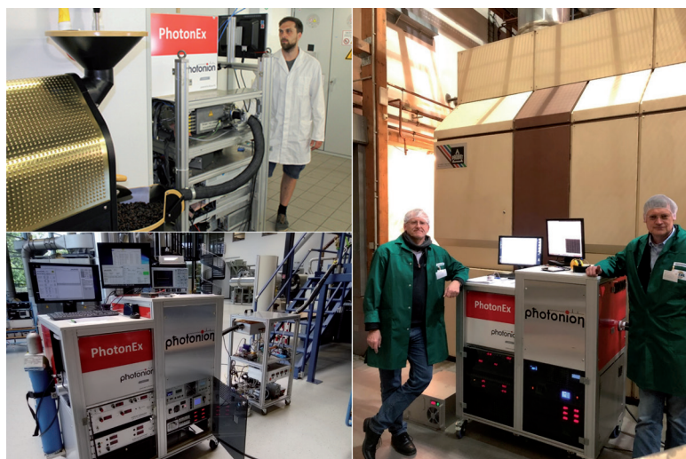
Figure 1: Coffee research scale-up from laboratory to industry using photoionization mass spectrometry for online investigation of coffee roast gases.
