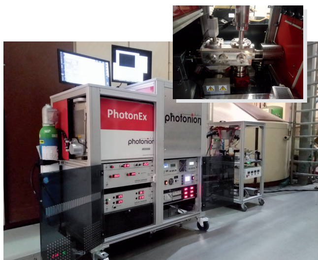
Figure 7: On-line gas-phase characterization. Dual on-line photoionization mass spectrometer (PhotoTOF; Photonion GmbH, Schwerin, Germany) for parallel acquisition of single-photon ionization using a VUV-lamp and resonance-enhanced multi-photon ionization (REMPI) mass spectra on a field campaign at the research laboratories of PROBAT-Werke von Gimborn Maschinenfabrik GmbH in Emmerich am Rhein.
