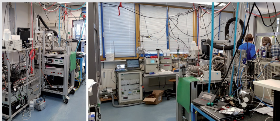
Some impressions of the first measurement campaign performed in at the HMHU in Munich: (Left) Mass spectrometers for online analysis of volatile organic components formed by aerosol aging (home build single-photon ionization mass spectrometer and a high resolution proton transfer reaction mass spectrometer). (Right) Aerosol sampling for off-line analysis and physical and chemical characterization of the secondary aerosol particles by scanning mobility particle sizer and counters and further aerosol mass spectrometry.
