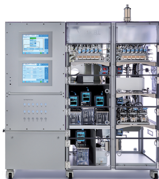
Figure 1: Automated exposure station from Vitrocell®. A versatile tool to assess in-vitro effects of aerosols at the air-liquid-interface. Exposures of up to 48 h were possible without increased cytotoxicity.
