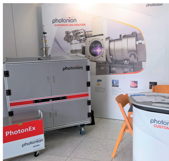
Figure 20: Photonion Booth at the European Aerosol Conference (EAC 2017) in Zurich, Switzerland. One of the latest Photonion products lines, based on a new Single Particle Mass Spectrometer (SPMS) concept is presented. Using a patented ion source, organic and inorganic chemicals can be on-line analyzed from individual aerosol particles in the size range from 150 nm-1 \mu m.
