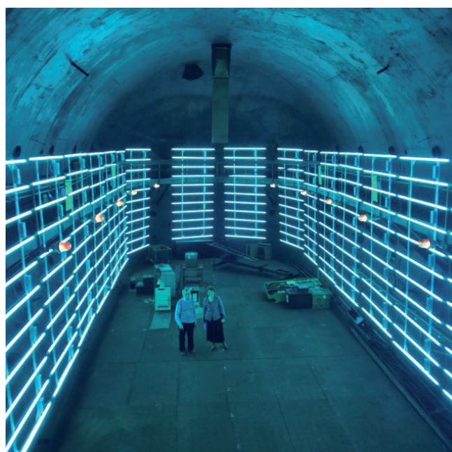
Figure 1: Realization of the illumination for the photochemical aerosol aging experiments in the LAC with 198 UV-lamps.
