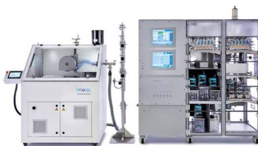
Figure 1: The newly developed cutting module (left) and the cell exposure unit (right) for the abrasive cutting experiments to assess the toxicological potential of particles released during the cutting process.
