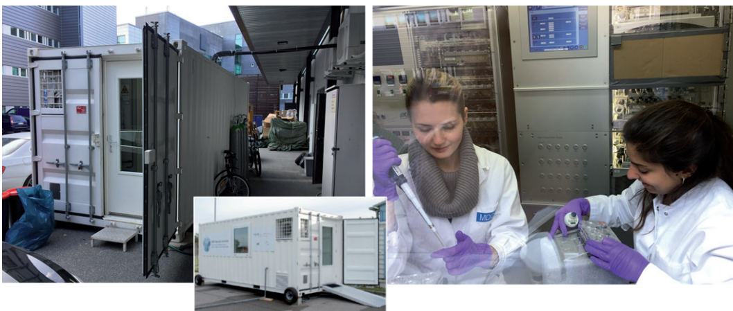
Figure 13: The HICE MobiLab, a mobile aerosol exposure and biosafety level 2 laboratory based on a 20 ft. shipping container. The HICE MobiLab contains two rooms. Left) HICE MobiLab in use at the University of Eastern Finland during a measurement campaign, the small insert shows the HICE MobiLab in Munich before shipping. Right) Photo of cell extraction and biological analysis work after cell exposures to wood combustion exhaust, taken through the HICE MobiLab window.
