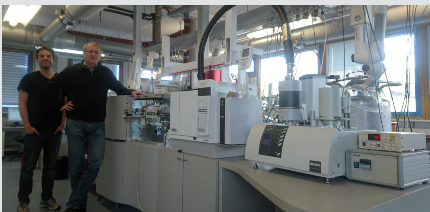
Prof. Zimmermann together with Dr. Uwe Käfer at the first LECO Pegasus HRT 4D System. The system is equipped with a direct insert probe, soft photoionization and a hyphenation for thermal analysis. Main applications will be the investigation of aerosols for the Helmholtz International Lab "aeroHEALTH".
