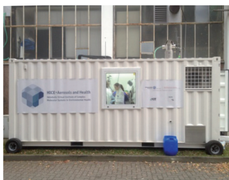
Figure 11: (left) The HICE-MobiLab during a measurement campaign for testing the biological activity and toxicity of shipping engine emissions (right) Mobile automated air-liquid interface (ALI) exposure station for direct exposure of cell culture and co-culture tissue models to aerosols.
