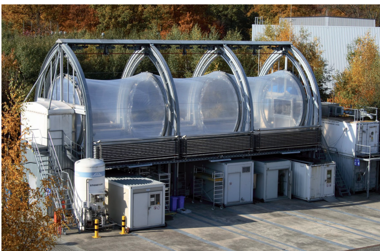
Figure 10: Aging experiments under realistic conditions can be performed in the SAPHIR aerosol chamber at the FZJ.
