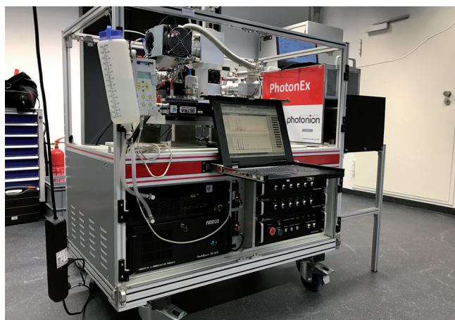
Figure 5: Aerosol Mass Spectrometry Lab. A single-particle mass spectrometer with advanced laser ionization technology developed in our group.
