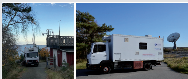
Some Impressions from the measurement campaign in Sweden: (Left) JMSC truck with single-particle mass spectrometer, measuring background aerosols in remote environment at the Swedish coast. (Right) Arrival at the measurement site in the restricted area of the Onsala space observatory.
